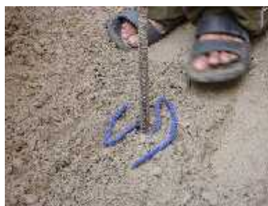
Direct Measurement of base sand depth
